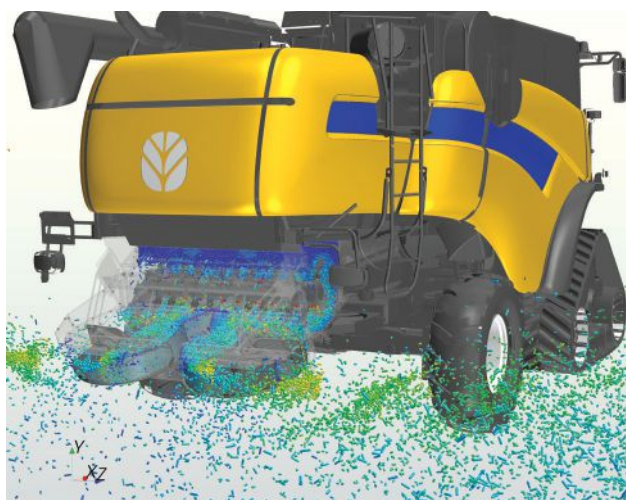
Illustration of the residue flow through the chopping and spreading mechanism of a New Holland combine harvester. The transient multiphysics simulation combines the DEM (discrete element method) and airflow capabilities of STAR-CCM+. Image courtesy of CNH Belgium N.V.
